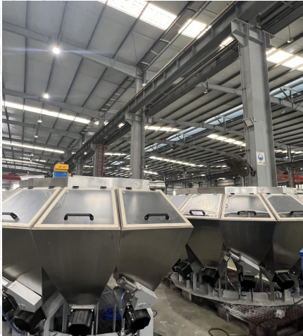
Multi-head Powder Weigher (Current Design applies glass lids, improve the airtightness)
