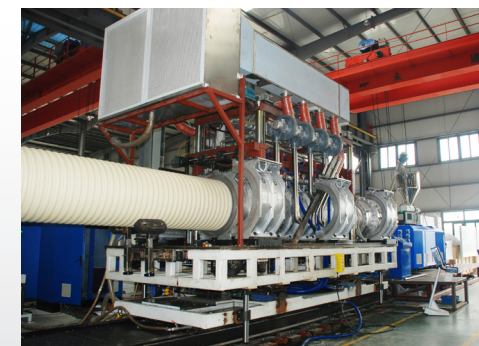
■ PVC 1000 double wall corrugator.
